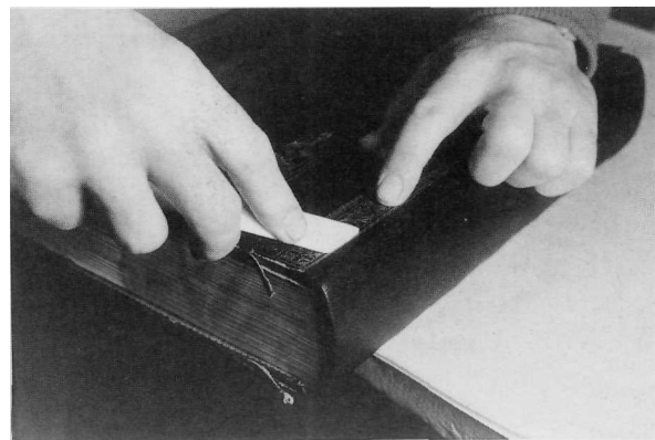
41 Feeding the leather hard up against the compensating strip.
