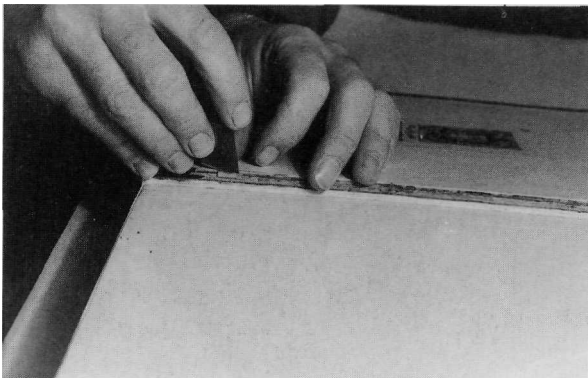
53 Removing the 0.6 mm card spacers.
