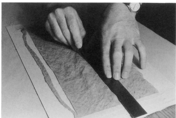
9 Unbleached Irish aeroplane linen is cut on the bias into strips (by cutting on the bias there is a 40 per cent increase in the number of threads running across the joint without adding any extra bulk). Unbleached cotton may be used for light-weight books. (See Phoenix advertisement)
