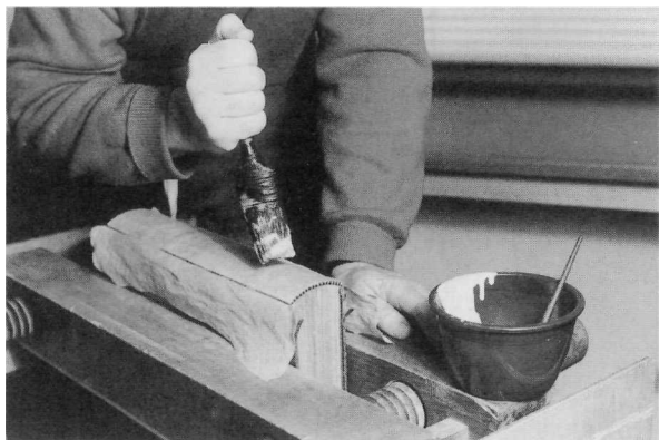
26 Gluing the spine and sticking the first linen joint across. If required, headbands can be sewn on through the linen after this stage.
